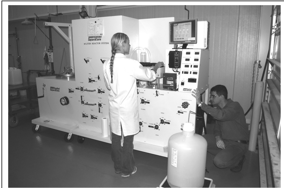
Figure 2. Research engineer Nestor Gonzalez and conservator Liisa Nasanen operating the second generation 40-L subcritical reactor.
